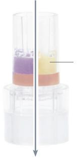
High definition colorimetric foam displays CO<sub>2</sub> level
