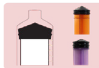
Rubber plunger tips are more conical, creating more surface area for unwanted lipid/fat adhesion.
