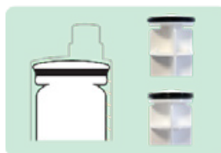
The solid polypropylene plunger head is flatter, creating less surface area for unwanted lipid/fat adhesion.
